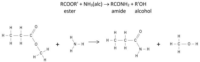
The reaction is slow, so the better method of forming amides is acyl chloride +  $NH_3$ (alc), RCOCl +  $NH_3 \rightarrow RCONH_2$  + HCl
