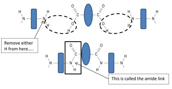
Polyamides can be hydrolysed under acid conditions  $(H^+/H_2O)$ .
